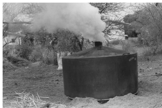
Figure 3: “3 barrel” kiln in operation
