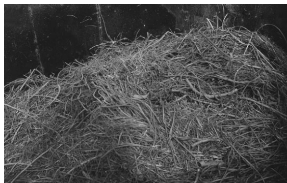
Figure 4: Carbonized Biomass, inside view of a “3 barrel” kiln
